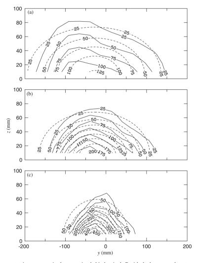
Fig. 9. The concentration contours in the yz section behind a single P with the buoyant exhaust gas. The x (mm) coordinate (origin at the vehicle head) is (a) -1775, (b) -1050, (c) -525. The solid lines are the measured data and the dashed lines are the optimal fit to the Gaussian form (6). Note that the contour interval is 25 ppm for (a,b) and 50 ppm for (c).
