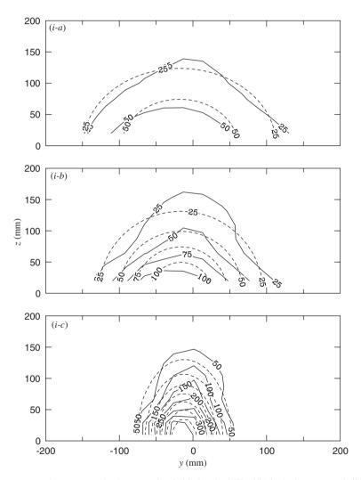
Fig. 10. The concentration contours in the yz section behind a single T with (i) the buoyant and (ii) the neutral exhaust gas. The x (mm) coordinate (origin at the vehicle head) is (a) -1829, (b) -1124, (c) -604. The solid lines are the measured data and the dashed lines are the optimal fit to the Gaussian form (6). Note that the contour interval is 25 ppm for (a,b) and 50 ppm for (c).
