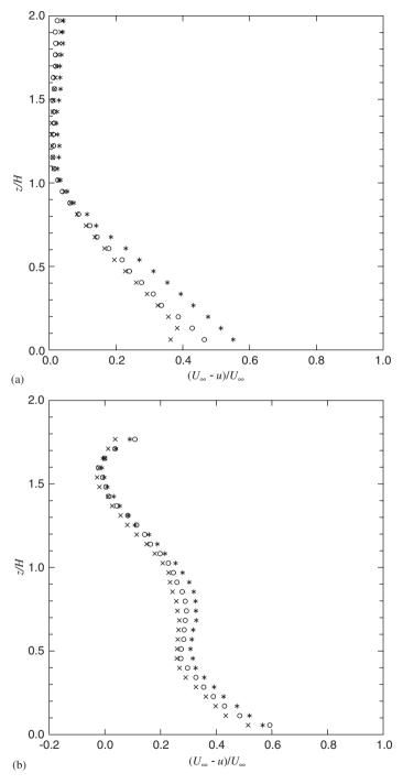
Fig. 7. Vertical profiles of velocity deficit for (a) P and (b) T. The normalized downwind distance x'/H from the rear end of the vehicles is (a) asterisk: 2.2, circle: 2.9, cross: 3.6; (b) asterisk: 3.7, circle: 4.4, cross: 5.1.  $U_{\infty}$  is the mainstream velocity.
