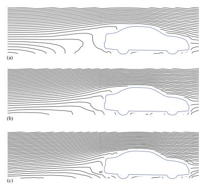
Fig. 4. Streamfunction contours at y = 0 around a passenger car (P) behind a queue of nine P's. The mainstream speed U (m s<sup>-1</sup>) is (a) 0.75, (b) 1.5, (c) 3.0. The contour intervals are proportional to U.
