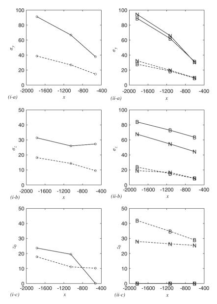
Fig. 11. The Gaussian fitting parameters  $\sigma_y$ ,  $\sigma_z$  and  $z_0$  for (i) the passenger car (P) and (ii) the truck (T). The units are all in mm. The dotted lines denote the results for the bare pipe experiments without the vehicle bodies. In (ii), the marks 'B' and 'N' represent 'buoyant' and 'neutral' gas, respectively.
