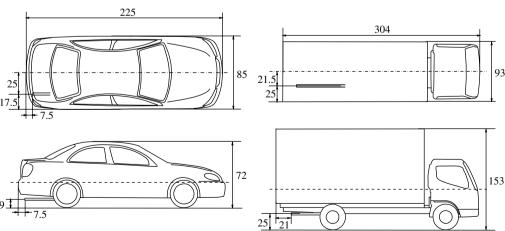
Fig. 2. Schematic drawings of the model vehicles. The unit of the length is mm. The shaded regions are the exhaust pipes. The dash-dot and the dashed lines indicate, respectively, the vertical and the horizontal sections for PIV measurement.
