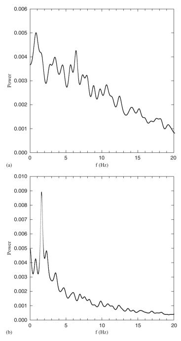
Fig. 8. Power spectral density distribution obtained from LDA data. The spectra are one-sided and are calculated by the maximum entropy method (lag =  $\sqrt{\text{number-of-data}}$ ). (a)  $(x, z) = (-265 \,\text{mm}, 25 \,\text{mm})$  (second row from the bottom, second column from the vehicle) behind P, (b)  $(x, z) = (-404 \,\text{mm}, 110 \,\text{mm})$  (fourth row from the bottom, third column from the vehicle) behind T.
