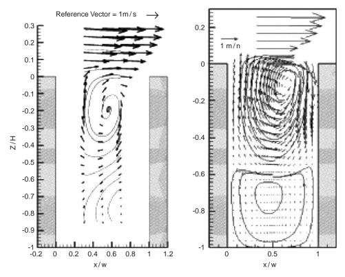
Fig. 5. Mean velocity vectors and stream traces on center-plane for W/H = 0.5 [39].
