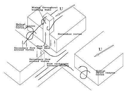
Fig. 6. Flow field at a street intersection [23].
