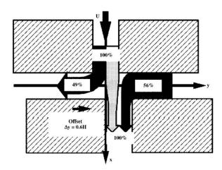
Fig. 7. Flow interchanges at an intersection defined by four blocks of height H, with a 0.6H off-set block size  $6 \times 4H$  [47].
