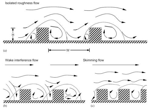
Fig. 3. Perpendicular flow regimes in urban canyons for different aspect ratios [27].
