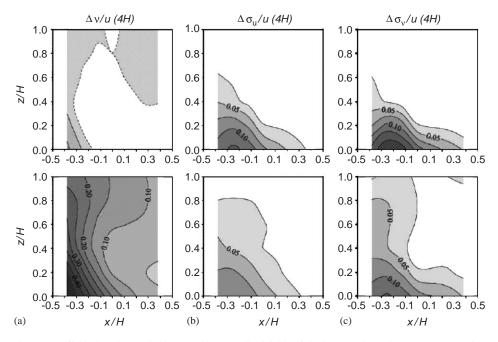
Fig. 10. Traffic-induced contributions to the normalized fields of the lateral (along-the-canyon) mean-flow velocity component (a), and r.m.s. values of longitudinal (b) and lateral velocity (c) fluctuations inside the 120 cm-long street canyon. The plots in the upper row refer to the case of two-way traffic and the lower row corresponds to the case of one-way traffic [71].
