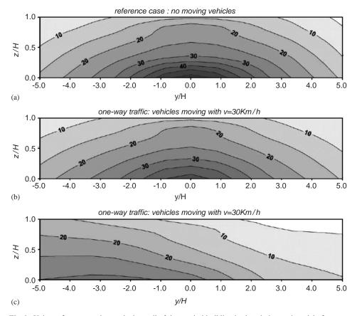
Fig. 8. Values of concentration at the lee wall of the upwind building in the wind tunnel model of a street canyon without traffic (a), with two-way traffic in opposite directions (b) and one-way traffic (c) [70].
