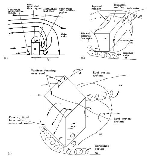
Fig. 1. Main features of flow around cuboids at 0° and 45° to the approach flow in a deep boundary layer [23]. (a) Mean streamlines on centre of a cuboid normal to the approach flow. (b) Mean flow pattern around a cuboid normal to the approach flow (lines marked 'sa' are mean separation/attachment lines). (c) Mean flow pattern around a cuboid at incidence to approach flow.
